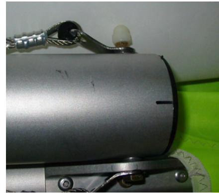
Nylon nut cap installed above clinch nut
