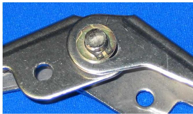
Originally, the center hinge fastener in this assembly was an NAS 623 517 Bolt and 5/16 Clinch Nut. In the spring of 2002, we switched to a combination of a 4C-37 Clevis Pin, a 5/16" Pushnut, and a safety ring for the center hinge pin in this assembly (pictured above, on left). In late 2004, we switched this assembly again to a grooved 5/16" clevis pin and a snap ring retainer (pictured above, on right.)
