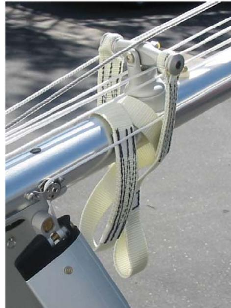
After mid May 2006, T2's were made with the same, 2<sup>nd</sup> configuration support pillar, but with a new, one piece spreader bar with integral end caps, and a new type of hang loop which fits tightly over the integral end caps and is then secured with plastic zip ties that pass through small webbing loops (picture on the following page shows the older T2 type spreader bar and hang loop on the left and the most recent, one piece spreader bar – hang loop assembly on the right).
