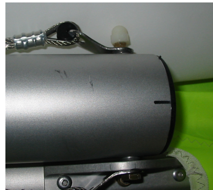
Nylon nut cap installed above clinch nut
