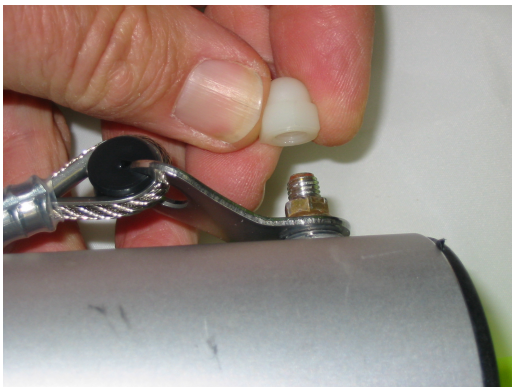
Installation of clinch nut
