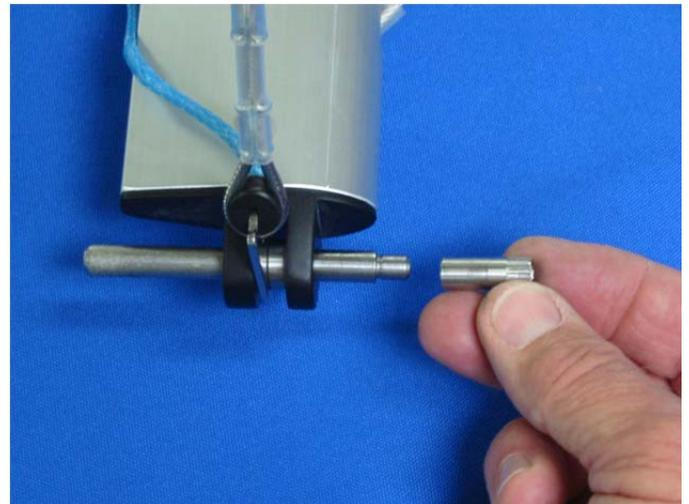
Reverse the sidewire bushing tool and press or gently tap the knurled bushing into the downtube plug until the end of the bushing is just flush with the surface of the plug, as in the second photo below. If the bushing protrudes, as in the first photo below, it will be difficult to assemble the downtube to the basetube bracket.
