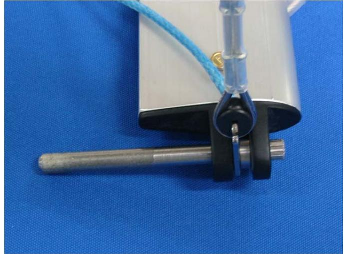
Using the sidewire bushing tool as a guide, and working from the back of the downtube plug to the front, assemble the components, including the new sidewire, in the order shown in photo #2 on the first page. Make sure to insert the sidewire bushing tool with the stepped end toward the front of the downtube end plug. Take care to install the side wire tang in the correct orientation, as shown.
