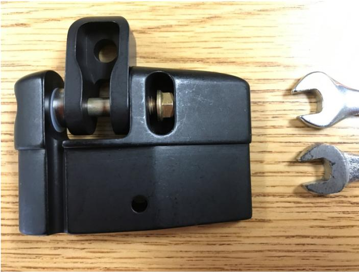
Route the upper VG rope around the inside of the bearing and through the slot in the downtube plug, and re-attach the pulley to the upper VG rope.
