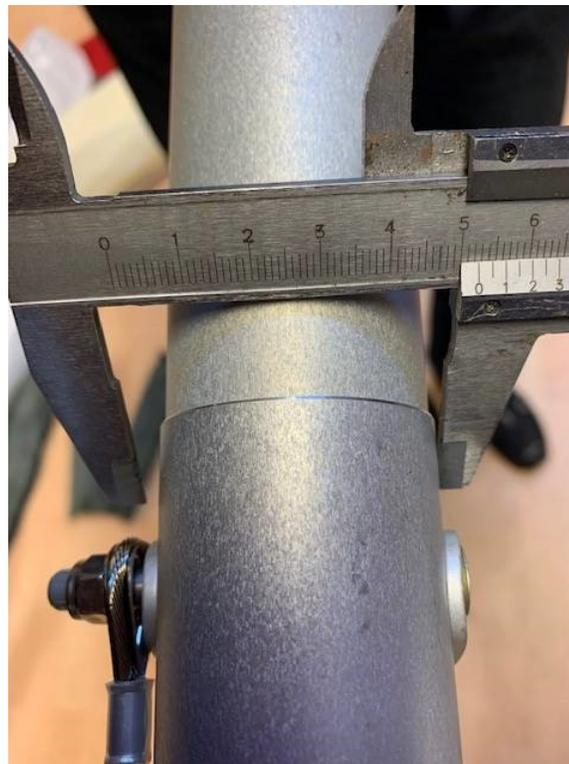
Sprog Bolt is overtightened, compressing the tube out of round
